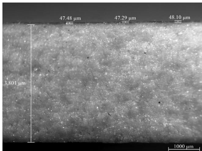
Figure 1. Stereo microscopy image of coating thickness at different parts on ceramic tile.
