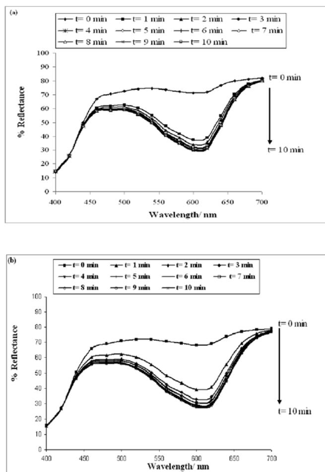
Figure 5. Reflectance spectra of coated ceramic tile under sunlight (a) and UV lamp (b) irradiation at different times.
