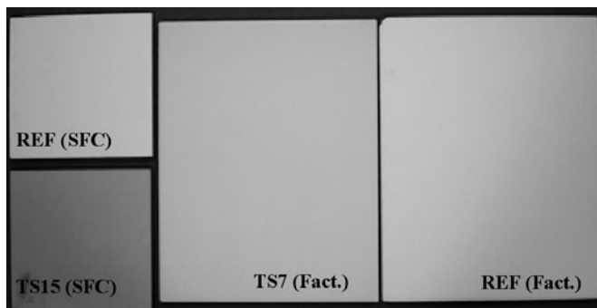
Figure 3. Appearance of non-glazed tiles (Ref. TS7 and TS15)
