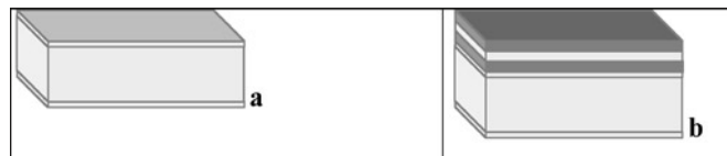
Figure 1: Scheme of the green coated structures used to fabricate the laminates.
