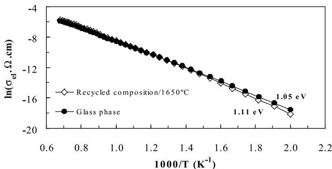
Fig. 5- Arrhenius-type plots of the mullite-based recycled sample, pre-sintered at  $1650^\circ\text{C}$ , and of the synthetic glass having the same chemical composition (estimated by EDS) of the intergranular glassy phase present in the recycled bodies.
