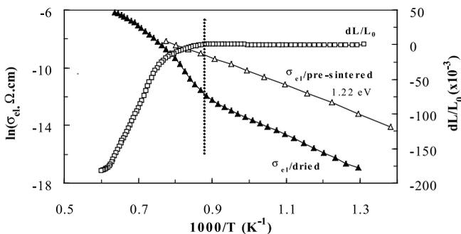
Fig. 4- Dilatometric curve ( $dL/L_0$ ) of dried mullite-based recycled sample and Arrhenius-type plot ( $\sigma_{el}$ , estimated by IS) of the same composition dried and pre-sintered at  $1350^\circ\text{C}$ .
