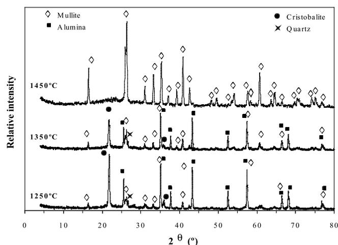
Fig. 7- XRD patterns of powdered samples sintered at three different temperatures for 1 hour.
