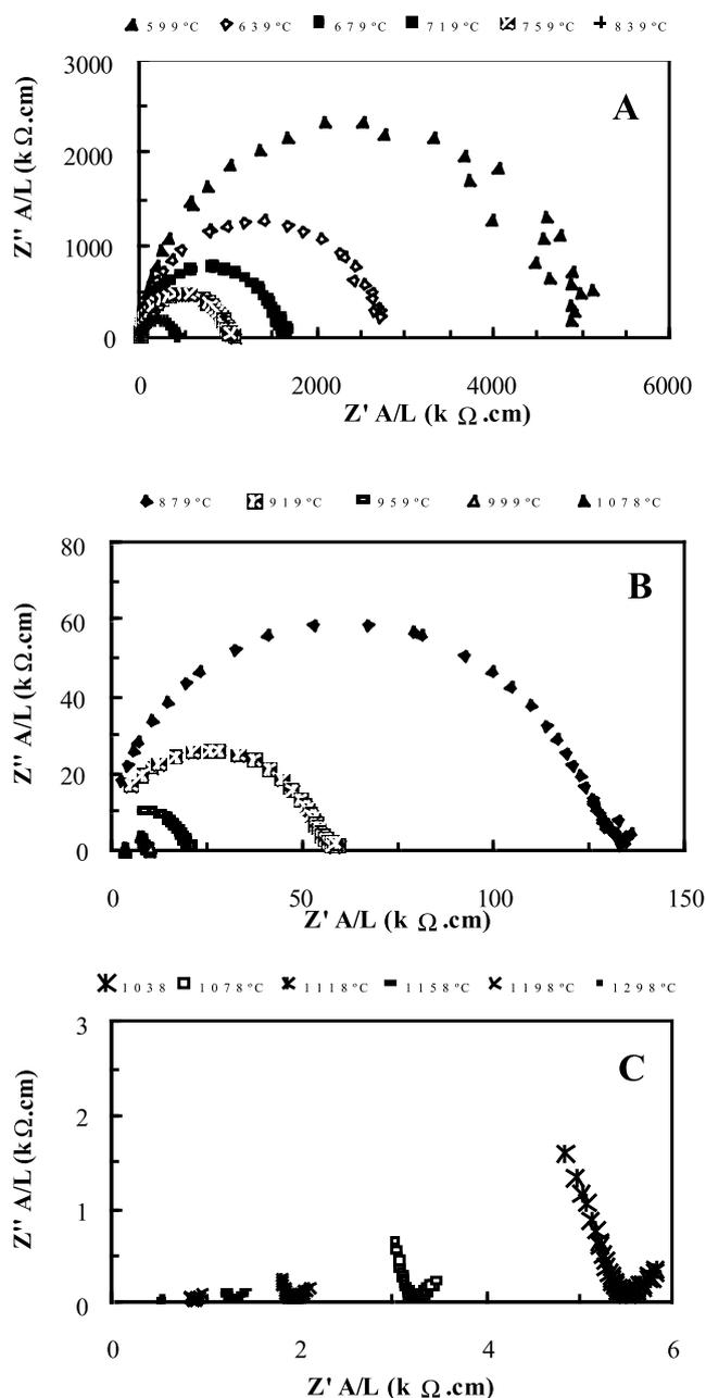
Fig. 3- Impedance spectroscopy evolution with the sintering temperature of extruded and dried mullite-based recycled samples.
