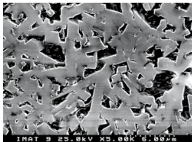
Fig. 6- Typical microstructures of mullite-based recycled samples: (a) sintered at  $1250^\circ\text{C}$ ; (b) sintered at  $1650^\circ\text{C}$ . In this sample the intergranular region was covered by the glassy phase, being mostly removed by chemical etching.
