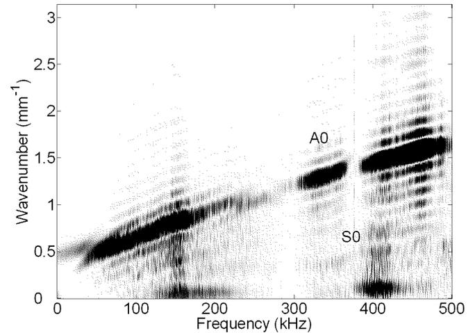
Fig. 6- Reinforcement of the antisymmetric Lamb mode and cancellation of the symmetric one by exciting the two actuators out of phase.
