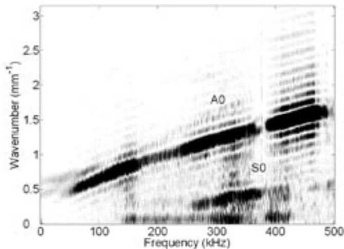
Fig. 4- Detailed part of the symmetric and antisymmetric modes showing the frequency region of interest of the experimental dispersion curves.
