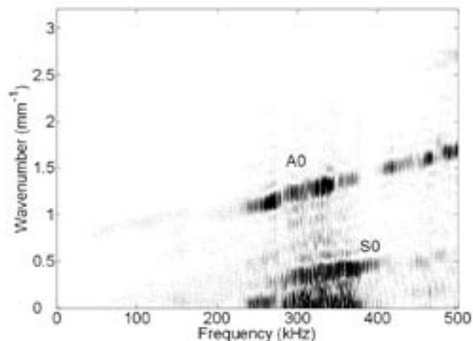
Fig. 5- Reinforcement of the symmetric Lamb mode and cancellation of the antisymmetric one by exciting the two actuators in phase.
