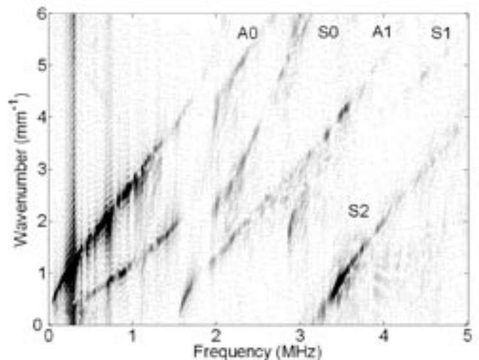
Fig. 3- Experimental dispersion curves for an aluminum plate of thickness 2h calculated applying the 2D FFT algorithm to the data measured with the needle hydrophone.
